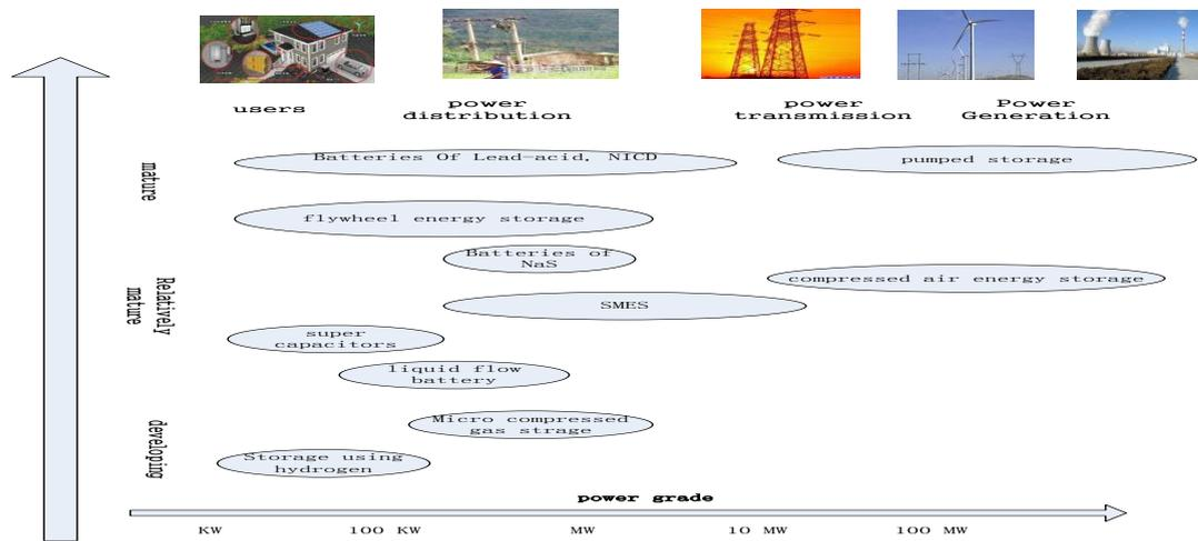
Fig.3 technical capability and commercial availability of energy storage types
